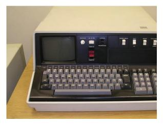
Another machine to have received attention in the last month was one of our two 5110 Desktop Computers from 1978. This was IBM's first all-in-one machine, with a small CRT display and able to run Basic or APL.
